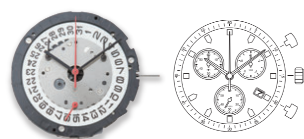
6S30 Height 4.90mm Chrono min / sec, 1/20 second 4 year battery life (SR927W)
