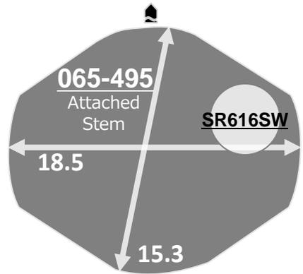
Battery consumption could be minimum by pulling out the stem
