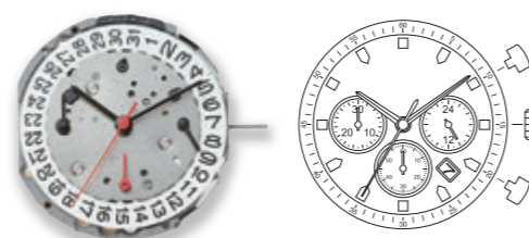
JS25 Height 4.30mm Chrono 30min/sec, 24 hour 3 year battery life (SR621SW)
