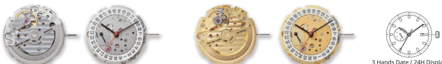
8217 Height 5.67mm / 21 jewels 21600 vibrations per hour Stop second device Automatic and hand winding Quick date setting
