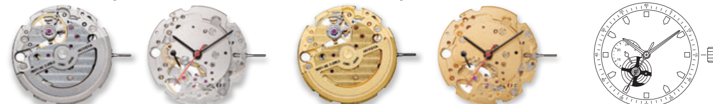
8253 Height 5.67mm / 21 jewels 21600 vibrations per hour Stop second device Automatic and hand winding
