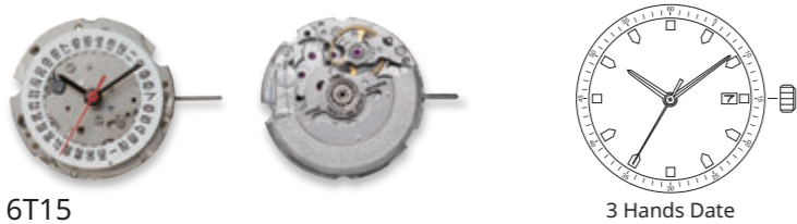
6T15 Height 5.98mm / 21 jewels 28800 vibrations per hour Automatic and hand winding Quick date setting
