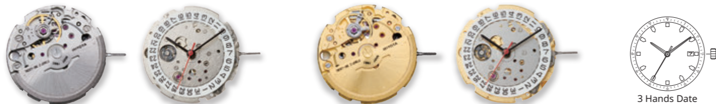
8215 Height 5.67mm / 21 jewels 21600 vibrations per hour Stop second device Automatic and hand winding Quick date setting
