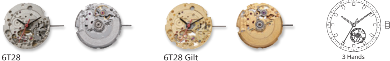
6T28 Height 5.23mm / 21 jewels 28800 vibrations per hour Automatic and hand winding Open-Heart
