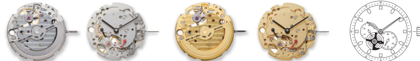
8257 Height 5.67mm / 21 jewels 21600 vibrations per hour Stop second device Automatic and hand winding
