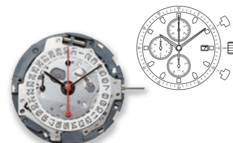
OS60 Height 4.13mm Chrono hour / min / sec, 1/20 second 2 year battery life (SR927W)
