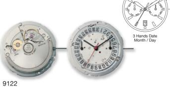
9122 Height 5.52mm / 26 jewels 28800 vibrations per hour Stop second device Automatic and hand winding Quick date setting
