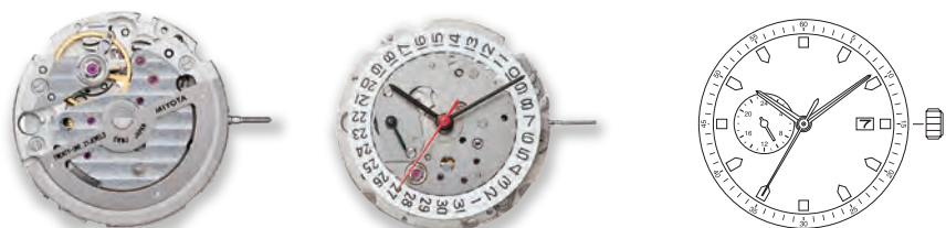
8217 Height 5.67mm / 21 jewels 21600 vibrations per hour Stop second device Automatic and hand winding Quick date setting
