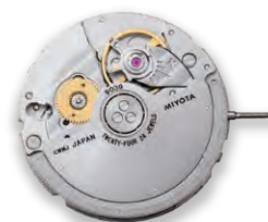
9039 Height 3.90mm / 24 jewels 28800 vibrations per hour Stop second device Automatic and hand winding
