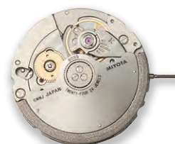
9055 Height 3.90mm / 24 jewels 28800 vibrations per hour Stop second device Automatic and hand winding
