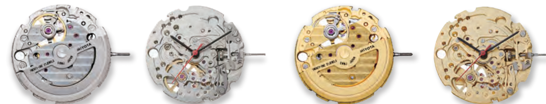
8250 Height 5.67mm / 21 jewels 21600 vibrations per hour Stop second device Automatic and hand winding
