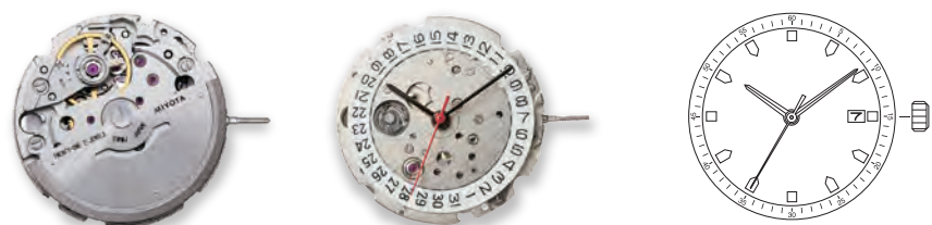
8215 Height 5.67mm / 21 jewels 21600 vibrations per hour Stop second device Automatic and hand winding Quick date setting
