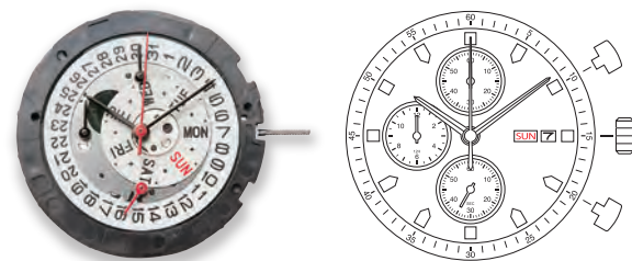
OS00 Height 5.10mm Chrono hour / min / sec 5 year battery life (SR927W)
