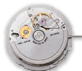
9100 Height 5.52mm / 26 jewels 28800 vibrations per hour Stop second device Automatic and hand winding Quick date setting
