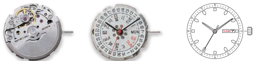
8205 Height 5.67mm / 21 jewels 21600 vibrations per hour Stop second device Automatic and hand winding Quick day / date setting
