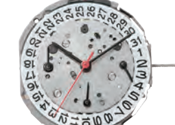
JP25 Height 4.30mm Day/Date/24 hour(3H) 3 year battery life (SR621SW)
