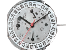
JP15 Height 4.30mm Day/Date/24 hour(12H) 3 year battery life (SR621SW)
