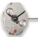
1L45 Height 2.93mm Small second: 6.61mm from center 3 year battery life (SR621SW)
