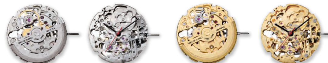
8N24 Height 5.55mm / 21 jewels 21600 vibrations per hour Stop second device Automatic and hand winding
