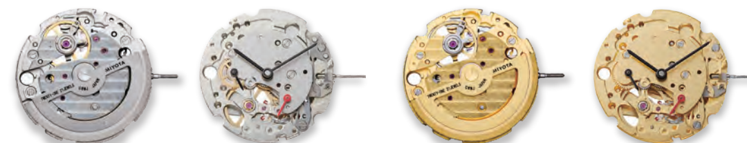
8257 Height 5.67mm / 21 jewels 21600 vibrations per hour Stop second device Automatic and hand winding
