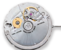
9015 Height 3.90mm / 24 jewels 28800 vibrations per hour Stop second device Automatic and hand winding Quick date setting
